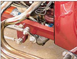
**Like the Vega gear, Corvair boxes can be used in cross-steering applications, but they are more often seen in T-buckets. In standard configuration, the Pitman arm points up.**
