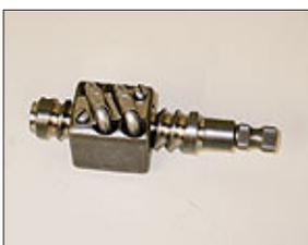
This is the worm and nut from the new Flaming River gear. Compared to the GM original design, this box has larger and stronger compo-
