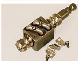
Here's the heart of a recirculating-ball steering gear. The balls fit between the threads of the worm and nut, which serves two purposes: they
