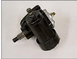
**Housings for these new boxes are made of cast steel. They're thicker and stronger than the originals and still weigh just 6 lbs.**
