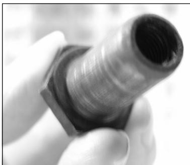
Pictured above is a close-up view of the replacement idler pulley adjusting nut fabricated from a rocker arm stud bolt. In this view you can see the inside threaded part of the adjusting nut. Elvis King made several of these replacement nuts to show at our Tuesday ACC meeting on January 17.
