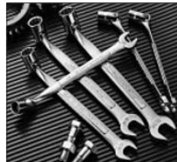
Pictured above is a set of Sear's Craftsman standard Saltus wrenches. The wrench is a cross between an open-end and a socket-end tool. The socket end pivots and can attack fasteners from more angles than possible with a standard 15-degree offset combination wrench.
