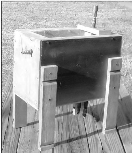
Above photo shows side view of the home-built drier (for compressed air) crafted from scrap materials by Elvis King. Note the air connections (inlet and outlet) at the left and top, respectively. Also, note drain tubing beneath. Photo at left shows a top-down view of manifold (copper tubing) inside the cooling box that holds chilled water to promote condensation. This device has yielded good results at low cost for Elvis.
